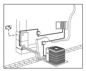
Fig.1—Typical Split-System Installation
